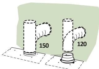
When installing the ducted version, connect the hood to the chimney using either a flexible or rigid pipe ø 150 or 120 mm, the choice of which is left to the installer.
