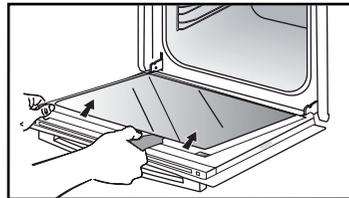
The door consists of two additional glass panels, with a black rubber spacer at each corner.
